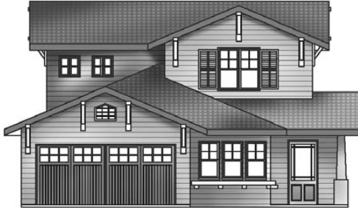
Style and materials of new second-story windows match and appear compatible with the original first -story of the house.
