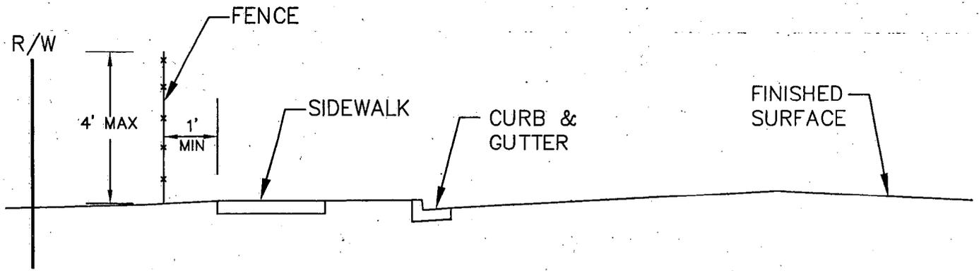
Fence Location Relative to Existing Sidewalks or where there is Evidence of Sidewalks
