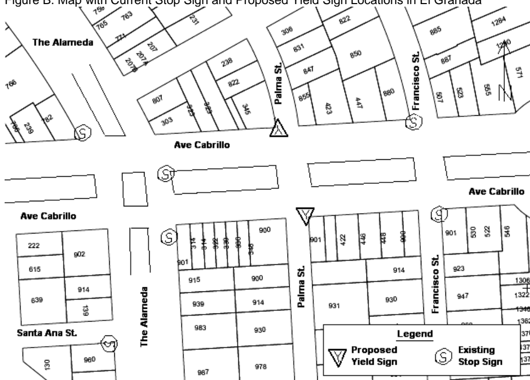
Figure B. Map with Current Stop Sign and Proposed Yield Sign Locations in El Granada
