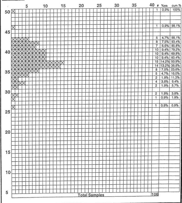
40.9 85th Percentile Speed: 36.9 50th Percentile Speed: 15th Percentile Speed: <u>33.8</u> 34- 43
