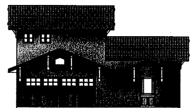
This second story located only over the garage appears out of balance..
