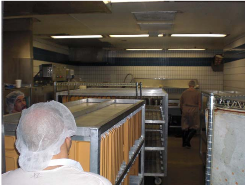
Dishroom is very tight and dishwasher needs to be replaced with electric flight type - $100,000
