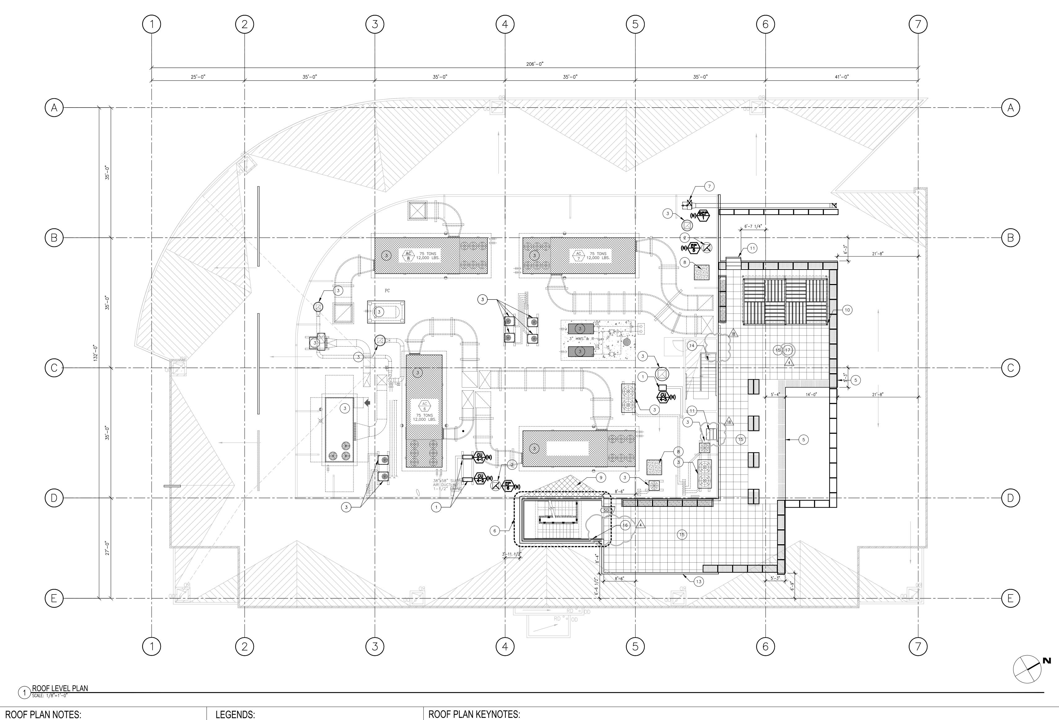
I ) (N) ROOFTOP CONDENSING UNIT ON EXISITNG SLEEPERS. REFER TO MECHANICAL DRAWINGS FOR MODEL,
